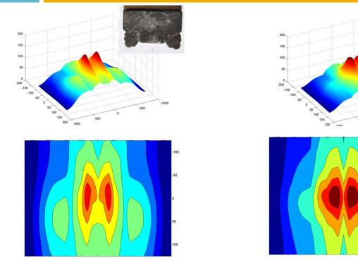
Nozzle 100.638.30.24 Water flow 2.2 l/min Air pressure 0,2 MPa
