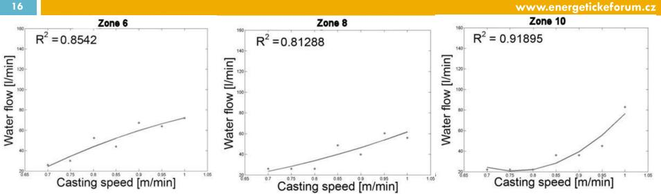
The optimal relationship between casting speed and cooling intensity.
