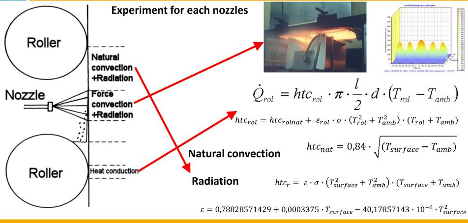
htc [W.m<sup>-2</sup>.K<sup>-1</sup>] heat transfer coefficient *I*, d [m] roller dimensions ε [-] emissivity
