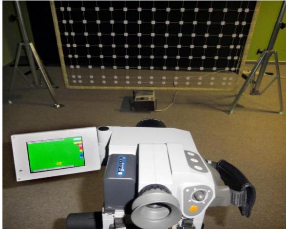
Fig. 4 The equipment for measuring temperature fields in 3D airstream
